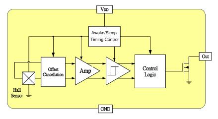
Note: Static sensitive device; please observe ESD precautions. Reverse  $V_{DD}$  protection is not included. For reverse voltage protection, a 100  $\Omega$  resistor in series with  $V_{DD}$  is recommended.
